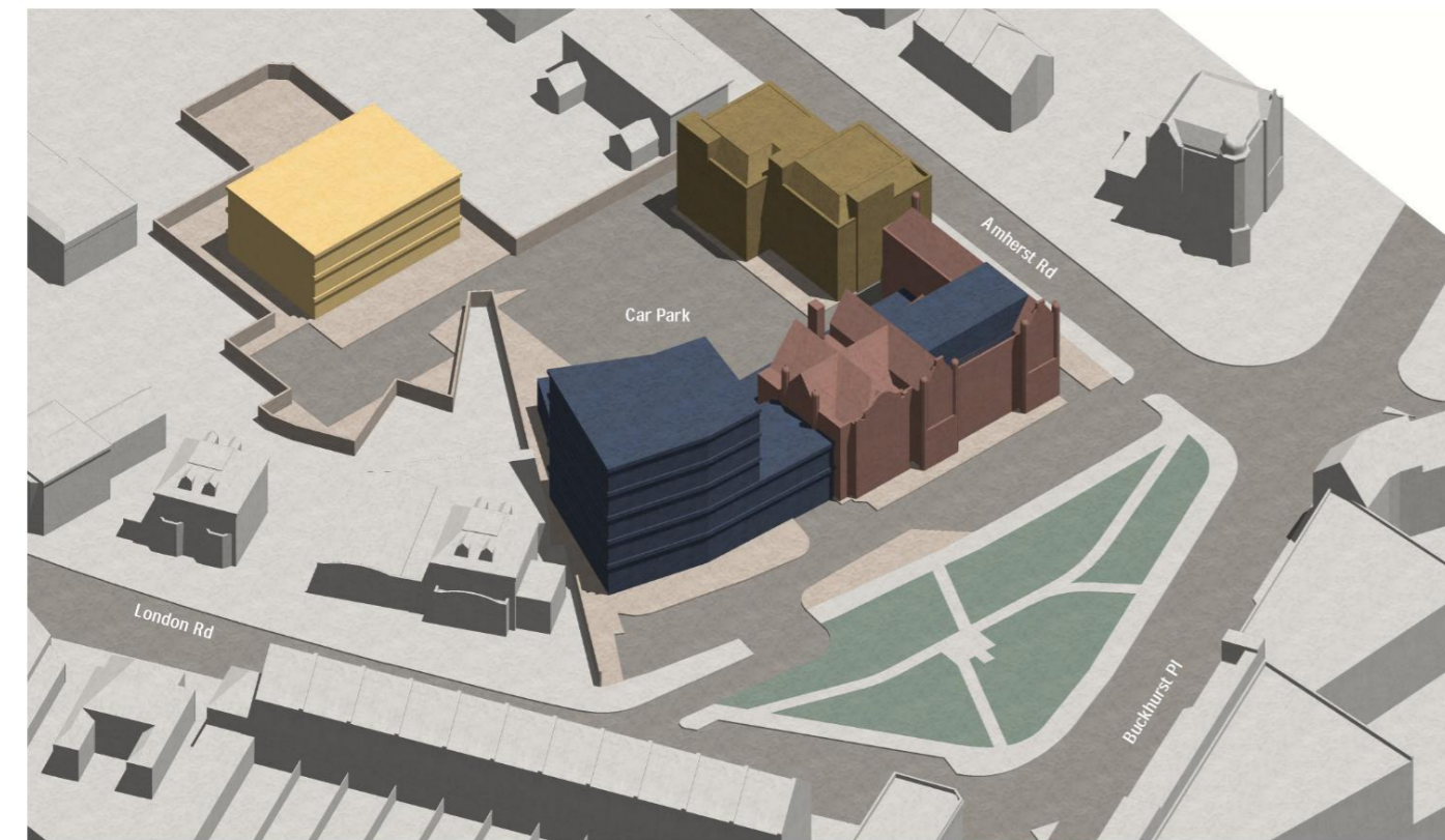
PROPOSED OPTION A Existing Town Hall building retained and refurbished/adapted Demolition of low quality rear parts, demolition of western converted houses. Proposed new commercial building Comprising of office space over 5 floor levels. Proposed new residential building Comprising of flats over 3 levels. 4 x 2 bed flats per floor = 12 x 2 bed flats total Existing building - Amherst Rd To be adapted and converted into residential units - Comprising of 4 x 1 Bed, 8 x 2 Bed & 2 x 3 Bed flats, 14 Flats total
