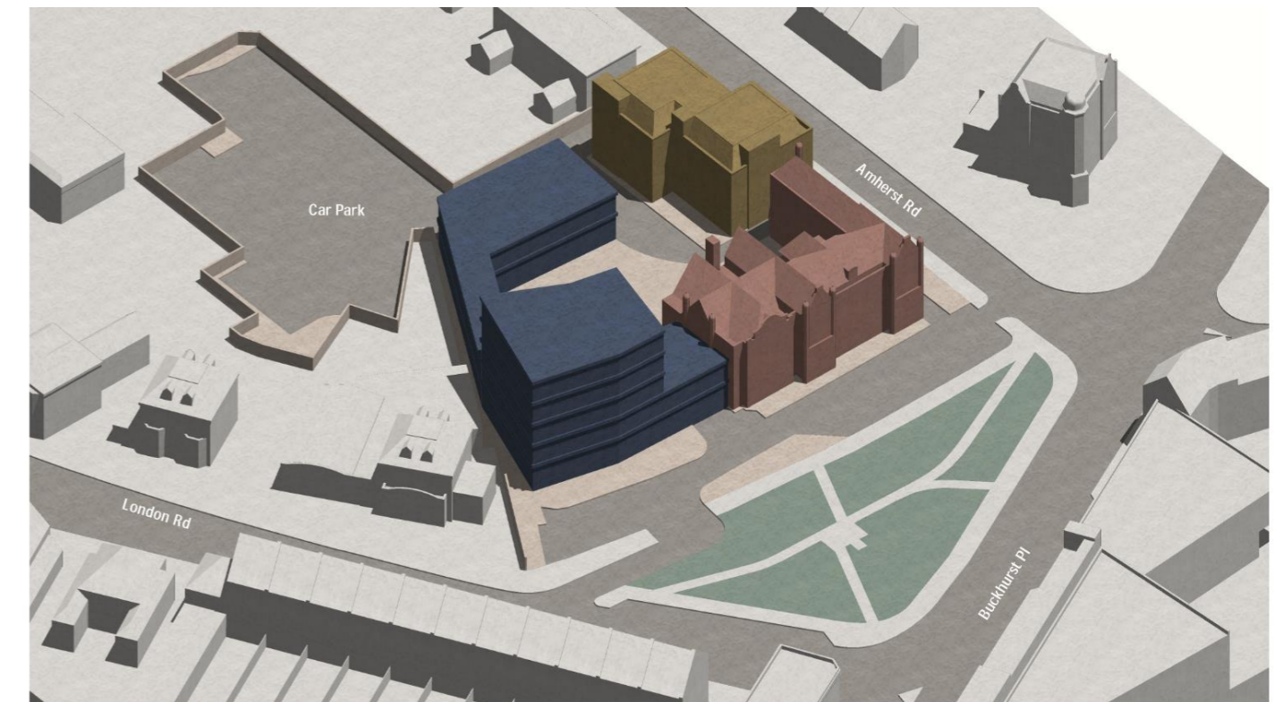
PROPOSED OPTION B Existing Town Hall building retained and refurbished/adapted Demolition of low quality rear parts, demolition of western converted houses. Proposed new commercial buildings comprising of office space over 5 floor levels on street front. Single storey rear western link. Two storey rear northern Commercial building Existing building - Amherst Rd To be adapted and converted into residential units - Comprising of 4 x 1 Bed, 8 x 2 Bed & 2 x 3 Bed flats, 14 Flats total
